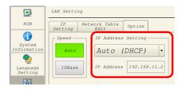
On V9, go to [LAN Setting] > [Option] > [IP Address Setting] and select [Auto (DHCP)].
