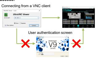
This is convenient such as for debugging because the remote screen is displayed immediately! Monitoring is possible without displaying the authentication screen on the V9 unit!
