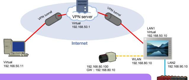
Routing function helps you to access to the Ethernet devices on the same network as V9's.
