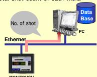
3) It's easy to check the maintenance timing of each mold on the list in real time.
