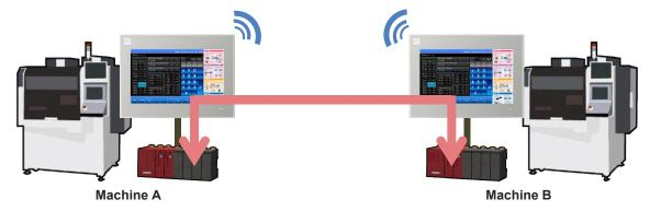
Quick action can be taken by sharing the alarm information of different machines. Hence, it helps shortening the down time and increase the efficiency of machine.
